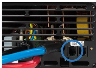
Connector is marked with ,Temp. Sense'.
