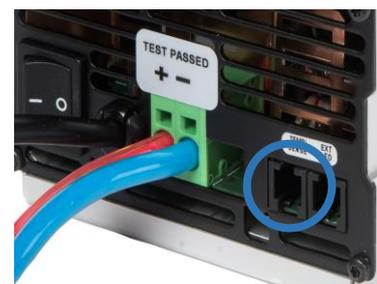
Connector is marked with ,Temp. Sense'. Older versions with only one connector: This is for the sense cable.
