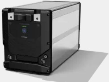
The 4th generation Lithium Power Pack is a module-based 12 V lithium iron phosphate battery (LiFePO4/LFP) that ensures reliable energy storage. Thanks to its high capacity of 280 Ah, it also fulfills demanding applications. The G4 series has an integrated battery management system (BMS) to protect the cells against deep discharge, overcharging and overheating.
