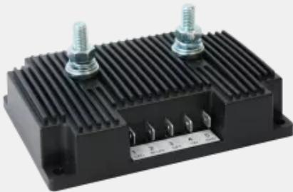
The CDR can be installed between the starter and auxiliary battery as an electronic battery isolator. The device can be used both bi-directionally and unidirectionally. The batteries are charged almost loss-free and the plastic housing protects against short circuits. Thanks to a switch-off function, it can also be used as a main switch to connect/disconnect a consumer or an on-board network.
